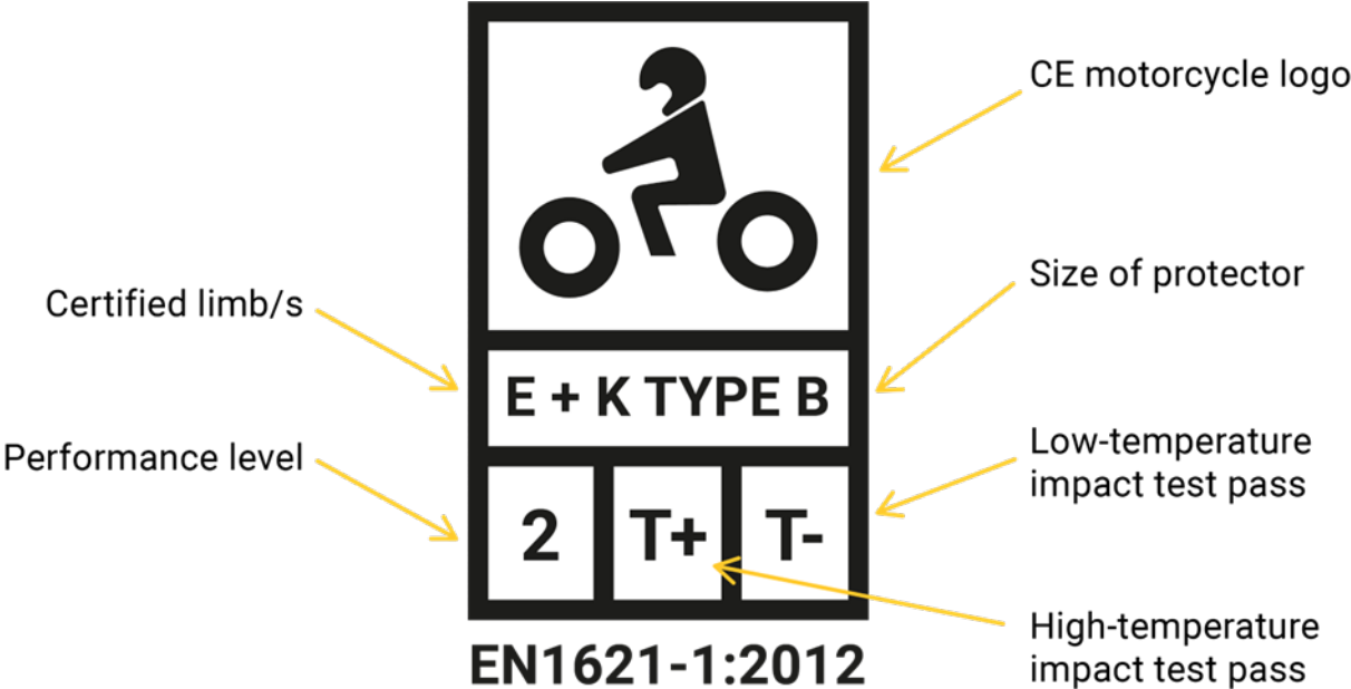
Figure 2.11: Description of the CE elements on the label of a limb impact protector.
